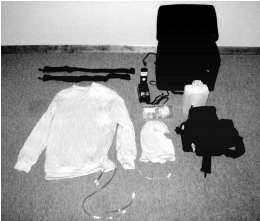
**Figure 2 - Core Control system used for the evaluation included, from top left clockwise: harness, battery charger, carrying case, 2 liter bottle, pump system hood, and shirt.**
