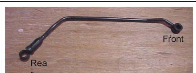
Figure 8. ATF bypass tube from the Ford Super Duty truck.
