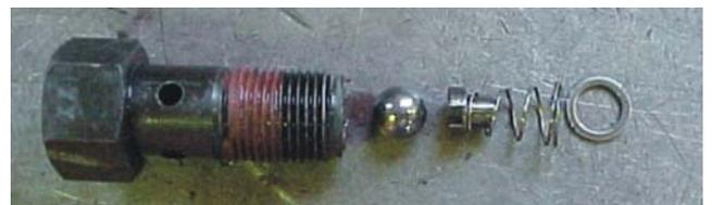
Figure 10. Cutting off the tip of the bolt allows removal of the check valve parts.
