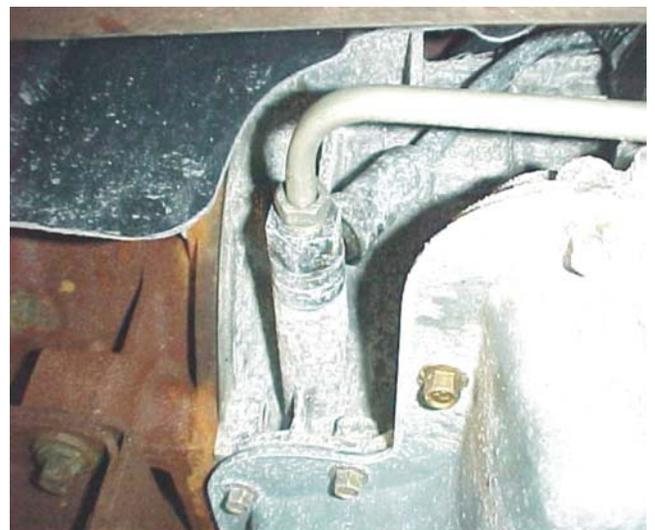
Figure 9. The ATF temperature relief ball valve, shown by the arrow and in Figure 10, closes when the oil temperature heats up sending the fluid through the coolers.
