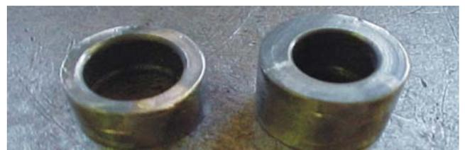
Figure 11. The spacers used to replace the bypass tube.
