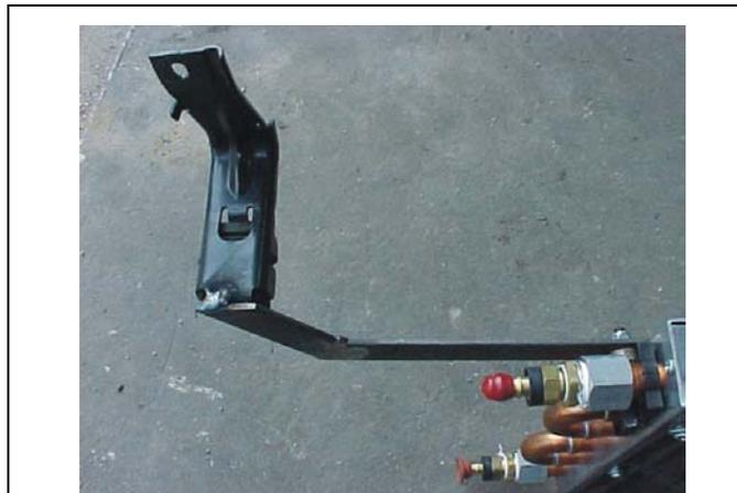
Figure 4. The factory stock radiator brackets were welded to the flat steel bracket to provide a mounting point for the cooler. Make sure that the bracket is solid enough to take some shock and vibration.
