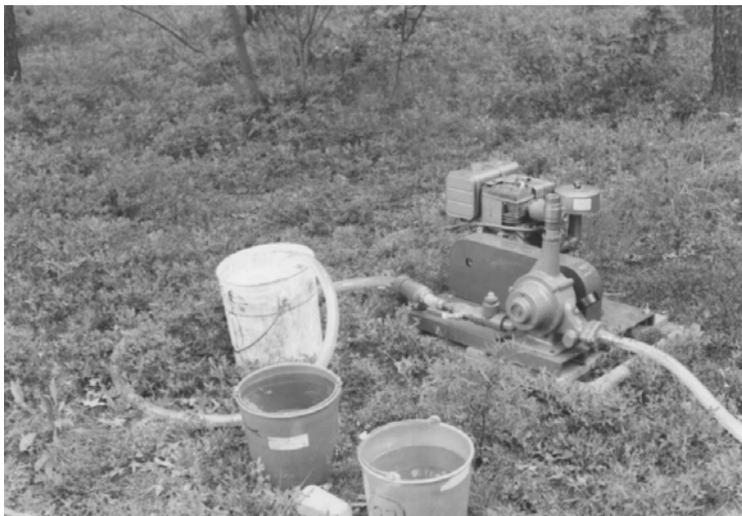
Expansion ratios vary from a high of 50:1 to a low of 7:1. The ratio is adjusted by changing the monitoring gear in the pump. The gear can be changed in the field by partially disassembling the pump. A field-adjustable expansion ratio changer could be added at extra cost.
