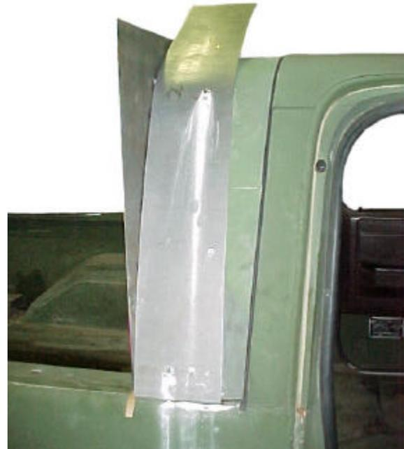
Photo 4 – The steel panel extension to the cab top is wrapped and bolted to the modified cap. The cap back can be used to locate it fore and aft.
