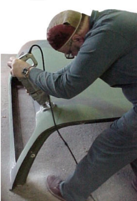
Photo 1 – The front of the cap is sawed off.
