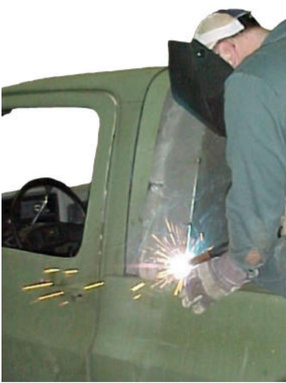
Photo 5 – The cap back panel is tack welded to the cap top extension. Once securely tacked together, remove the components to finish the welding process off the vehicle.
