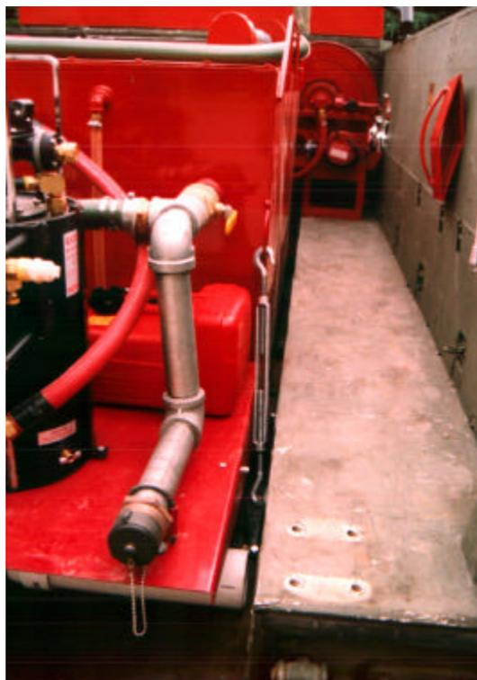
Figure B-3 - The tank is held in the cradles by four turnbuckles. The right rear turnbuckle is shown in the center of the photo. It is attached to the tank and to a cargo tiedown ring in the M548.
