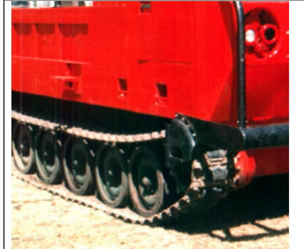
**Figure 3 - Removing the track guard step plates (shown installed near photo's center) reduces the overall vehicle width to under 103 inches. This eliminates the need for wide load permits.**
