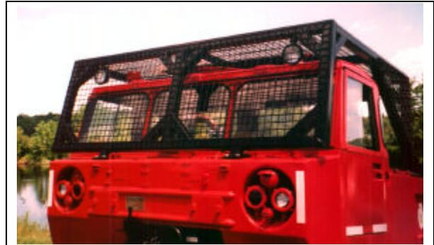
**Figure 2 - Windshield and cab protection on an M1015 unit produced by Maine Forest Service. The cab was a military composite material type with gun turret opening.**
