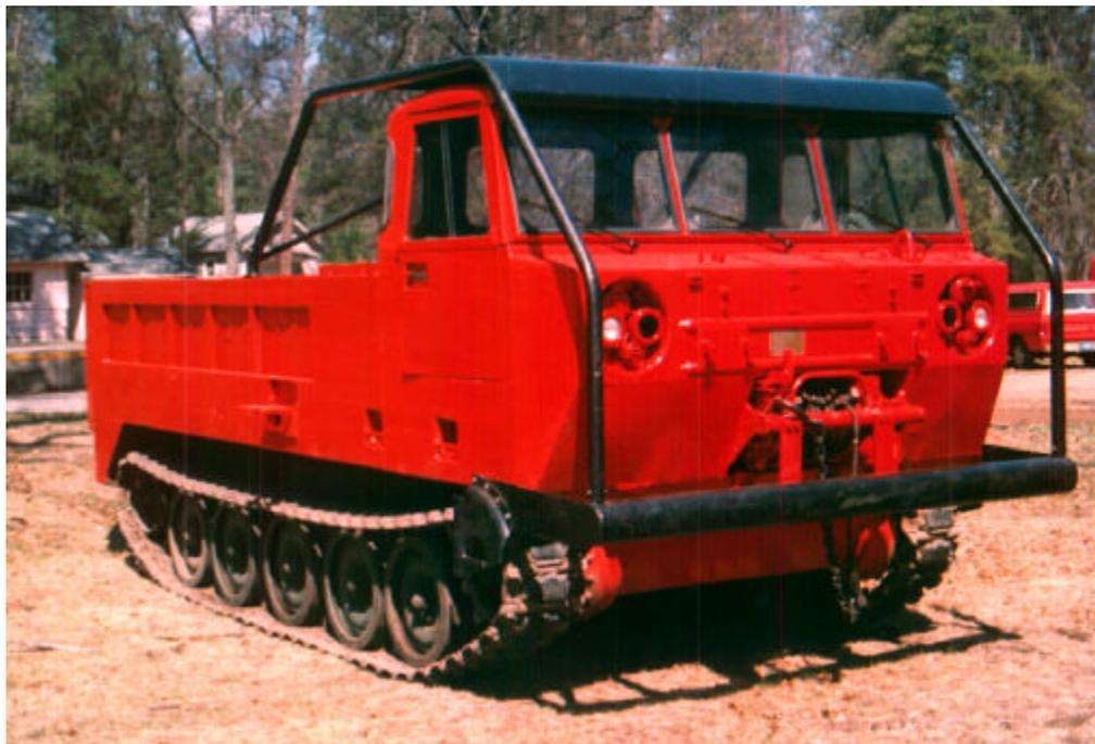
Figure B-1 - Front view of an M1015 modified by REC. Limb risers and bumper were part of the modification.
