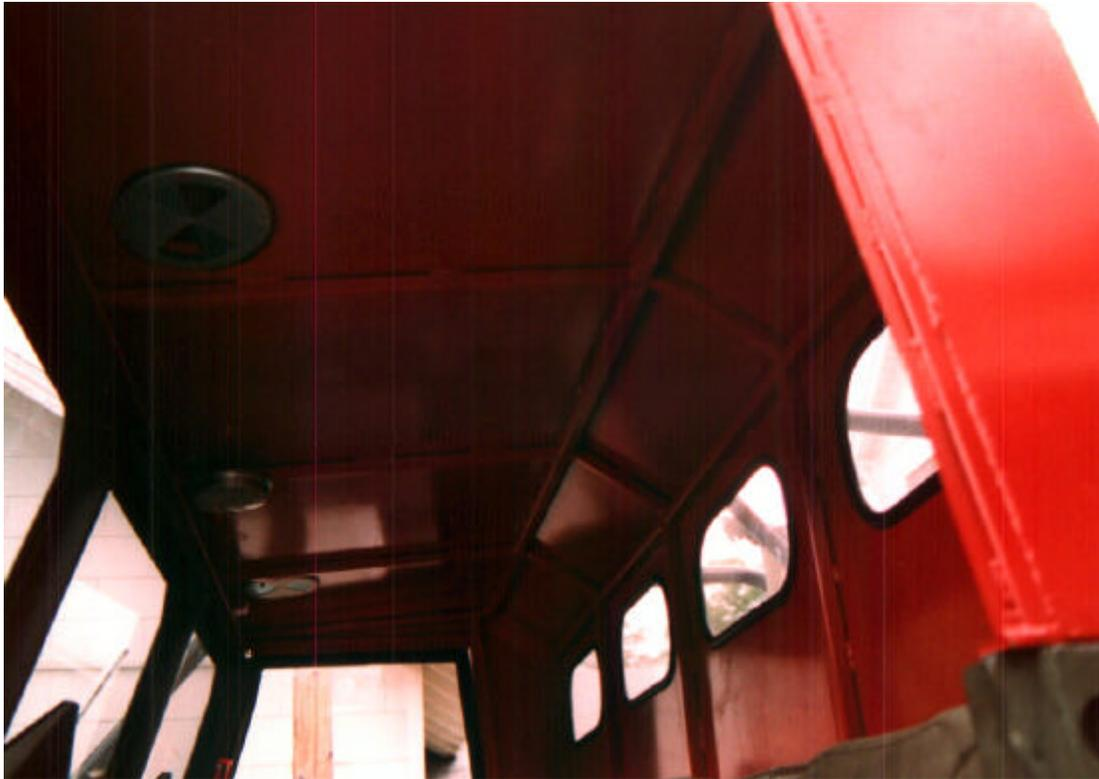
Figure B-5 - View inside of the REC cab. A 1x1 inch square tube framework supports the 11 gauge steel skin. The rear windows were a clear polycarbonate.
