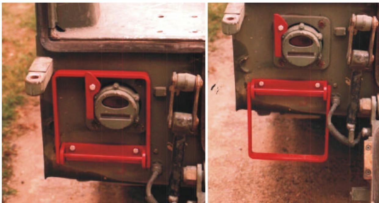
Figure B-8 - Fold down steps were put at each rear corner to reduce the step up distance to the cargo area (Design Packet #60E).
