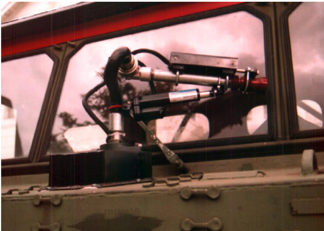
Figure B-7 - The REC low cost turret was integrated into the front of the M548 (see REC Project #58). The turret provides water delivery when it is not practical to use booster lines.
