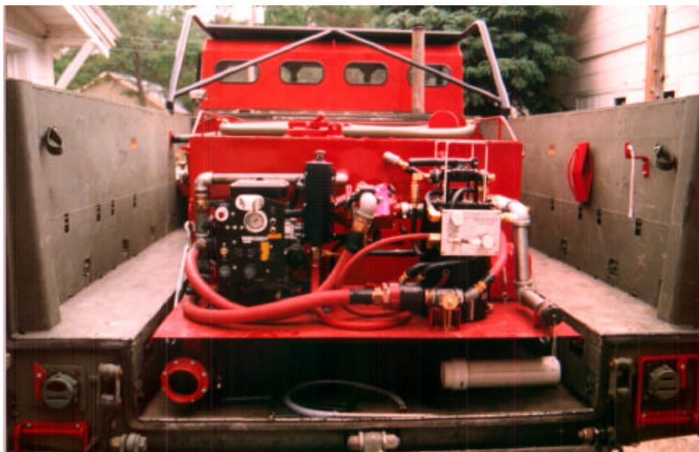
Figure B-2 – The 800 gallon REC tank with pump and foam proportioner. The tank sets in four cradles (not visible). Enclosed storage is located below the pump apron, accessed by opening the lower tailgate.
