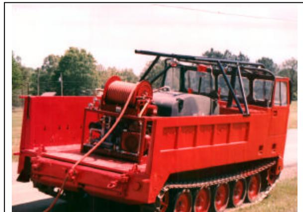
**Figure 1 - An M548 fitted with a military 500 gallon fuel cell and compressed air foam system (CAFS). Completed by Arkansas Forestry Commission.**
