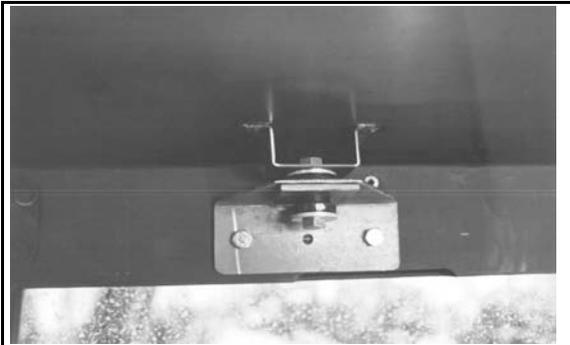
**Figure 2 -- The cab top mounting brackets were mounted to the windshield frame using two threaded insert nuts (33-0023). An isolator mount attached the roof to the cab top mounting bracket (35-0001).**
