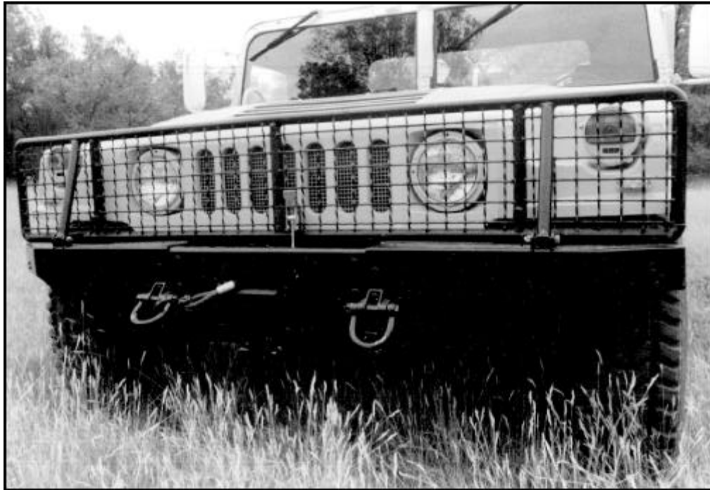
Figure 10 – Bumper extensions and a folding grill guard.
