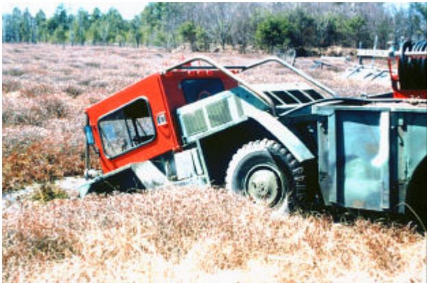
Figure 5 - The weight of cab top and brush protection can easily exceed the payload capability of the front axle. This is discussed in the report.
