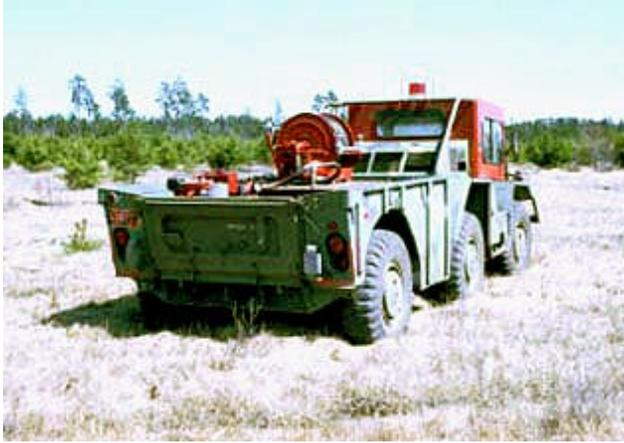
Figure 2 - If its front deck apron is reduced by four inches, the 200 gallon REC design M-715 slip-on tank fits into the Gamma Goat. It also loads the vehicle properly.
