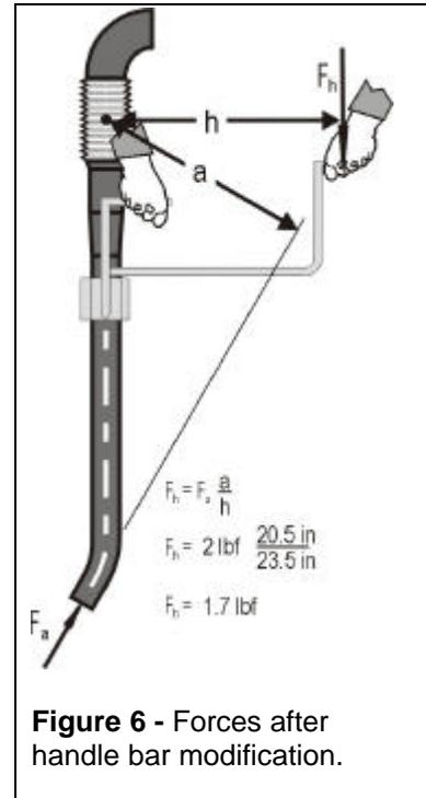
Figure 6 - Forces after handle bar modification.
