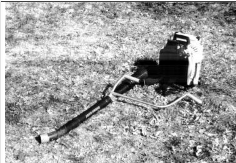
Figure 5 - REC Handlebar prototype with John Deere 5E blower.
